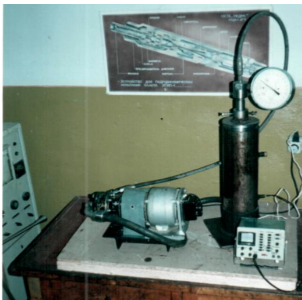
Fig. 3. Photo of the laboratory bench for studying the hydrodynamic pulsator operation
